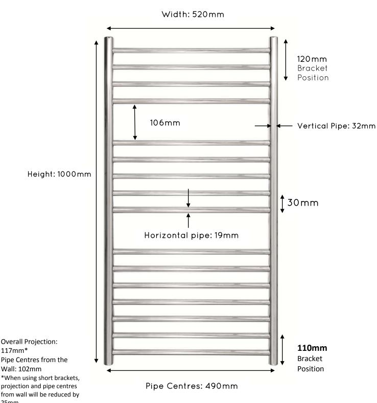
117mm\* Pipe Centres from the Wall: 102mm \*When using short brackets, projection and pipe centres from wall will be reduced by 25mm.
