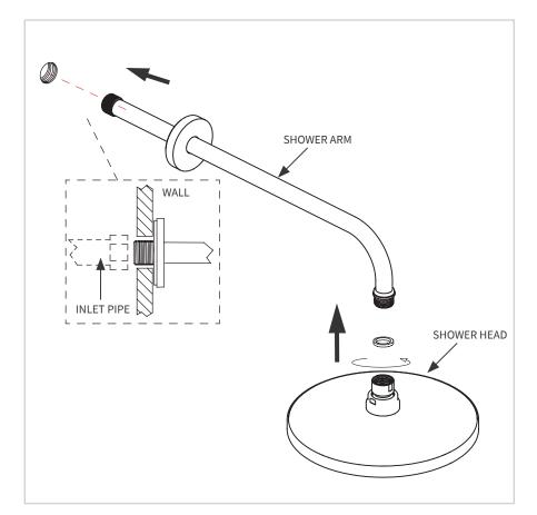
Install the shower arm using a suitable thread sealant
