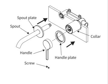
First shut off your water heating system, then with your mains stop cock closed, open the lowest cold and hot taps in the house and allow to run until the cold storage tank and pipes are empty (the hot storage cylinder always remains full). Fitting isolating valve to inlet feeds is recommended for ease of maintenance.
