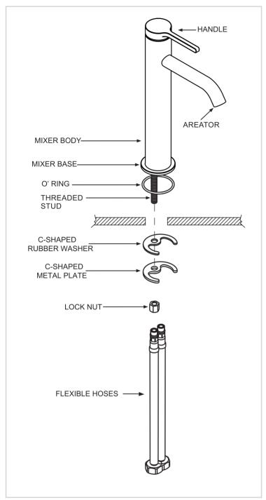
Screw the flexible hoses into the mixer body, and fully hand tighten. Place mixer in position to see if any alteration to the existing supply pipework is necessary.
