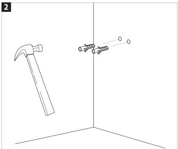
Place rawl plug in hole and use hammer lightly to ensure fully in the wall. Note: The fixing provided are for solid walls. For any other wall type, please use the appropriate fixing.
