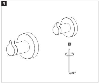
Place accessory over base on the wall and tighten the grub screw in place with a hexagonal key.
