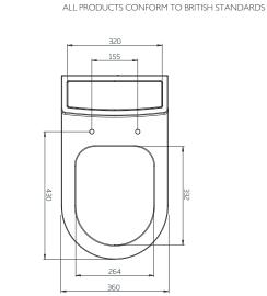
DIAGRAMS NOT TO SCALE | ALL DIMENSIONS IN MM TOLERANCE OF  $\pm$  5MM
