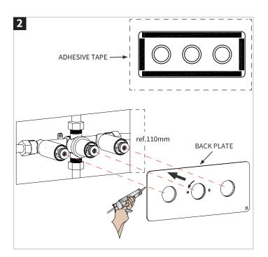
Remove the adhesive tape film on the backside of back plate.
