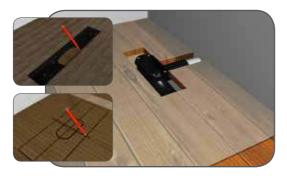
Measure the shower drain base position on the floor and mark this onto the relevant flooring. Using a jigsaw cut a hole in the plywood so that the shower drain base and shower drain connector will be exposed through the new floor.
