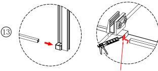
Add dab of silicone to the joint where luna rail and pivot bracket meet.
