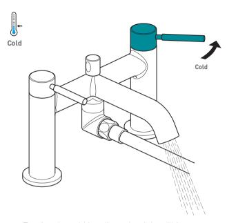
Turning the cold handle to the right will increase the flow of cold water.
