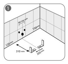
1 - Prepare the waste pipe and the fixing brackets according to the distances in the diagram.
