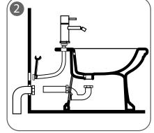
3 - Align the bidet and secure it with the fixing nuts.
