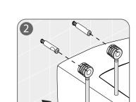
2 - Screw in the two steel sleeves located in the fixing pack
