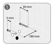
1 - Prepare the waste and the fixing rods as shown in the picture and cut if necessary
