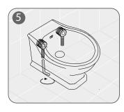
5 - Adjust the WC and secure it with the fixing nuts provided in the fixing pack
