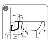
3 - Prepare the connection for the cistern flushing according to the given dimensions
