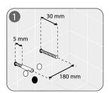
1 - Prepare the waste and the fixing rods as shown in the diagram. Cut if necessary.
