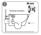
3 - Prepare the connection for the cistern according to the dimensions shown in the diagram. We suggest lubricating both sides to make the connection easier.
