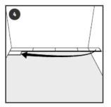
To create staggered joints, cut down the first tile of the second row. This should be a minimum length of 400mm.
