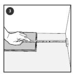
To measure up for the last tile in the row, place an 8mm spacer against the wall and measure the distance between the spacer and the previous tile.
