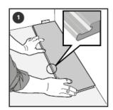
Start by laying your first tile in a corner of the space, with an 8mm spacer between its short end and the wall. Don't use spacers along the long edge at this stage.
