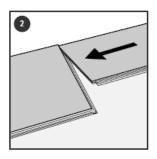
Place the short end of the second tile against that of the first tile, angling it into the locking strip and gently flattening it. Press gently on the joint between the tiles to seat them. Repeat this for the rest of the first row of tiles.
