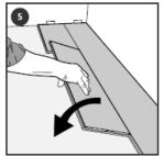
Place an 8mm spacer between the short end of this tile and the wall and slot the back edge of the tile into the locking strip of the first row tiles, holding it at an angle of approximately 30°. Slide it sideways until it meets the spacer, then fold it down and press it into place.
