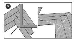
Cut the planks to this line, using a utility knife or a circular saw if possible. This should create two straight edges from which you can continue laying.
