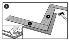
square to align the two planks perfectly. Then tap gently with a soft mallet to lock together.
