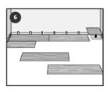
Attach the second plank by connecting the long side to the first row and sliding it up to the short end of the first plank. Check that the long joints of the planks are properly engaged and then press the short joint into place with your fingers.
