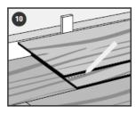
Most often the entire length of the last row will need to be cut so that it is narrow enough to fit the remaining space. Cut the first plank of the last row to length (if necessary to follow stagger pattern). Place directly on top of the previously installed row. Then, take another plank and place it against the wall on top of the plank to be cut for width. Mark the plank (lengthwise), and cut to size. Remember to allow for the 6mm expansion gap against fixed objects.
