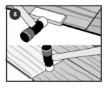
After installing the last piece of the second row, slide the entire assembly against the spacers on the starting wall, maintaining the required 6mm expansion gap.
