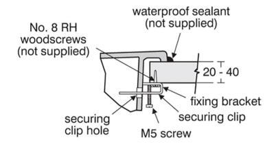
section through basin showing securing clip
