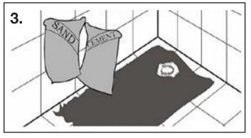
Ensure the installation base is completely solid and level with sand and cement mix. When the base is dry, place the tray with polymer or similar of aqueous base.
