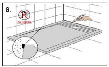
Seal between the tray and the wall with a silicone sealer and leave for 24 hours.
