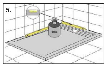
Level the tray ensuring there is sufficient water drainage
