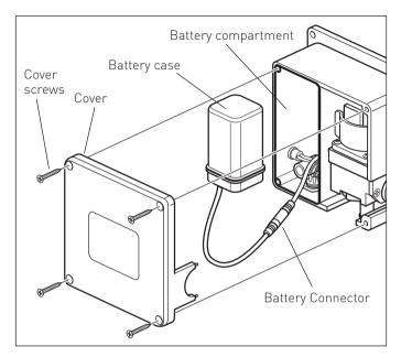
The unit is supplied with a battery backup, should the mains supply fail and the tap still will not function then the batteries may need replacing.
