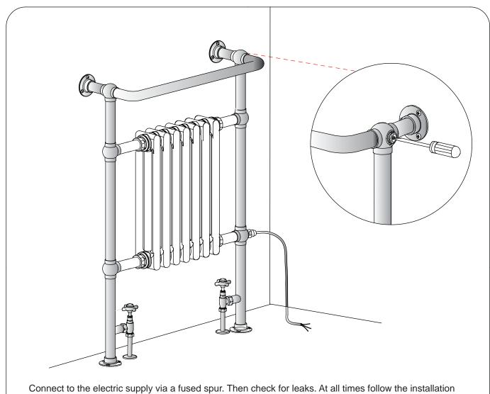
Connect to the electric supply via a fused spur. Then check for leaks. At all times follow the installation instructions supplied with the Summer Electric Heating kit. All electric work must be done by a suitably qualified person.
