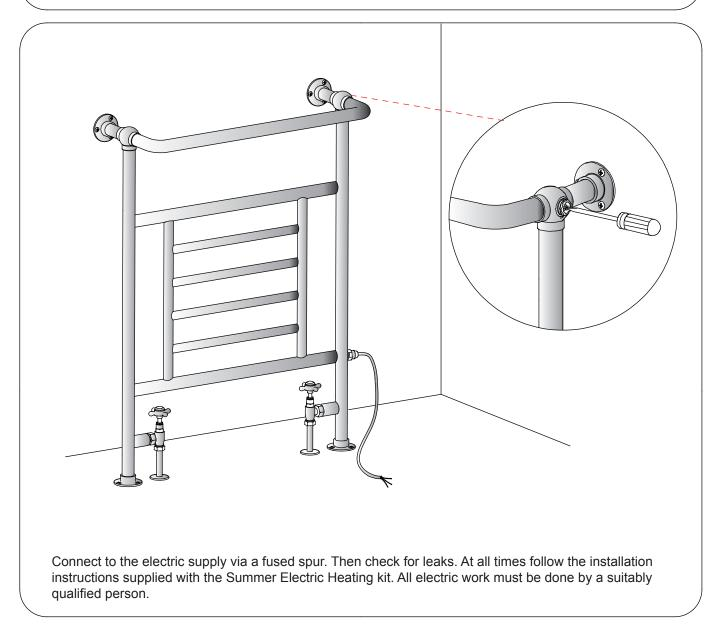
If this radiator used as a dual source connected to central heating system and with a summer electric heating kit fitted:
