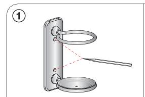
Determine the final installation position, mark the fixing hole positions in pencil.
