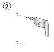
Using a 6mm drill bit, drill holes on the marked positions.
