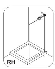
The side panel is reversible for left or right hand fitting, simply turn the panel up side down.
