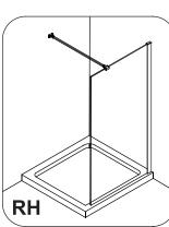
The side panel is reversible for left or right hand fitting, simply turn the panel up side down.
