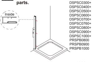
Get the wall channel from the packing. Place wall channel in position on the tray, use a spirit level to ensure that it is vertical and mark all 3 fixing holes onto the wall. We recommend the wall channel is placed not less than 10mm from the front edge of the tray.
