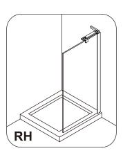
The side panel is reversible for left or right hand fitting, simply turn the panel up side down.
