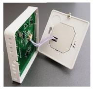
The connection lead can be disconnected on the screen circuit board if required by carefully removing the plug from the socket.
