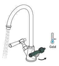
Turning the cold handle anti-clockwise will increase the flow of cold water.
