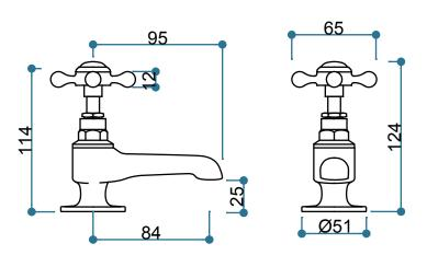
Identify the hot tap and position into the bath on the left hand, from the underside of the bath fit the rubber washer and then the nut. Making sure the tap is in the right position tighten the nut to secure the tap to the bath.
