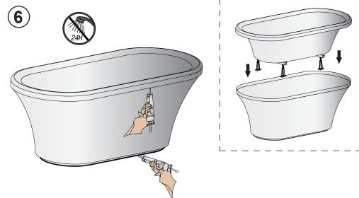
Once the overflow waste and taps have been fitted. The edge between the rim and the Surround should be sealed with a bead of clear silicon.
