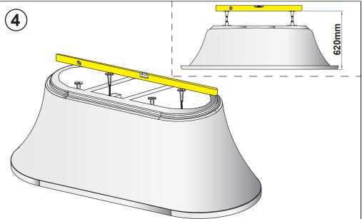
• Set the bath at the height of 620mm from floor to the top of the bath rim. Install the Surround on to the bath and adjust if required to ensure that the bath feet are level with the Surround in fitted position.
