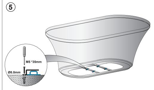
• All four floor brackets should face the same direction to allow the Surround to slide underneath during final installation.
