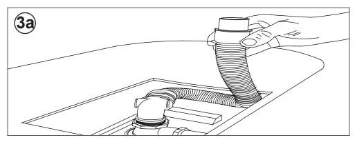
Method 1) If you have a waste that comes up through the floor, you can connect to it with a flexible drain pipe which enables you to tilt the bath up and move the bath into the required position. To avoid water retention in the trap the flexible pipe should have a continuous downward flow
