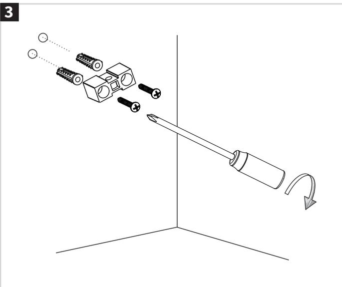
3 Align base holes with raw plugs in the wall and use a screw driver to secure in place.
