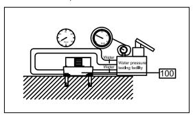
2.Make pressure test for the base union 100 by 10 hours in 10 bar to assure there is no any leakage befor the next step.
