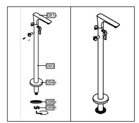
6.Put the covers 094 onto the pole 093 and mount the fixing round plate 098 onto the end of pole 093.Meanwhile fix thes pout 081 onto the body,locking with hexagonal spanner.
