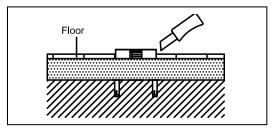
4.Pave the wood or gound tile and cut the exceeded part of the plastic box
