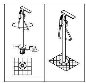
7.Take away the protective cover from the base union 100 and mount the poles 093 onto the base plate,locking with the nuts 097.Then slide down the cover 093 onto the floor
