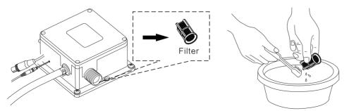
Clean filter: (1)Turn off isolating valve.(2)Unscrew flex hose.(3)Take out filter.(4)Wash filter out and replace.
