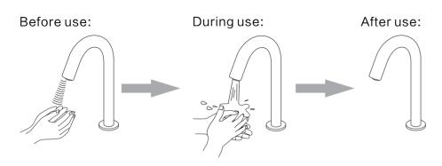
Note:when your hand enters the inductive field the water flows,remove your hand from the field and the water stops. It will stop automatically after flushing 30 seconds continuously, leave your hand from the inductive field for 3 seconds then enter the field to flush again.
