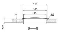
Note: Unless marked, the length, width dimension tolerance should be  $\pm 5$ . The tray thickness dimension tolerance should be  $\pm 2$ . The waste hole ID dimension tolerance should be  $\frac{4}{3}$ .
