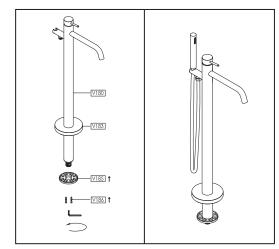
6.Put the covers V183 onto the pole V180 and mount the fixing round plate V185 onto the end of pole V180.
