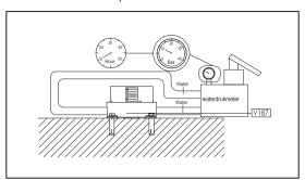
2.Make pressure test for the base union V187 by 10 hours in 10 bar to assure there is no any leakage befor the next step.
