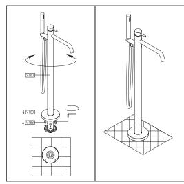
7.Take away the protective cover from the base union V187 and mount the poles V180 onto the base plate, locking with the nuts V187A.Then slide down the cover V183 onto the floor.
