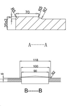
Note: Unless marked, the length, width dimension tolerance should be  $\pm 5$ . The tray thickness dimension tolerance should be  $\pm 2$ . The waste hole ID dimension tolerance should be  $^{+2}_{-3}$ .
