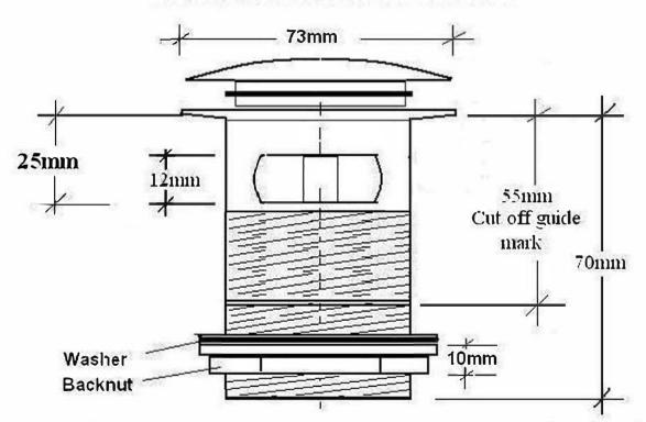
Marked as guide at 55mm in case the body needs length reduced
