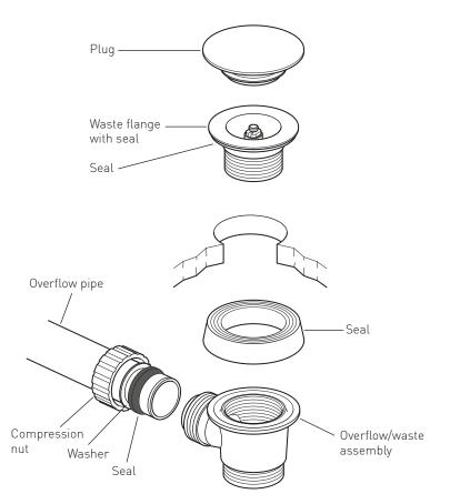
Push the seal onto the waste assembly
