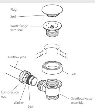
Push the seal onto the waste assembly
