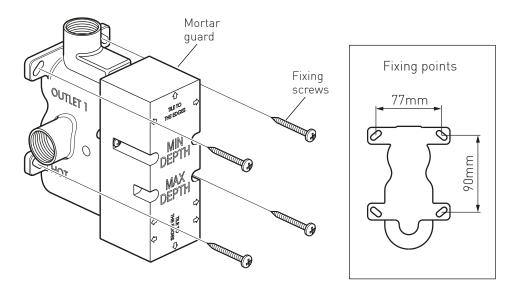
Select the position for the shower valve and offer the shower valve to the wall, make sure the valve is vertical with a level and mark the 4 fixing points with a suitable pencil, see above right for dimensions. Remove the shower valve from the wall, drill the holes to a suitable depth for the wall plugs and secure with suitable screws.
