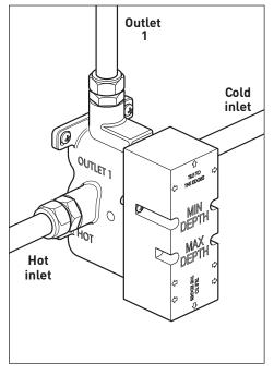
Finish the wall by tiling up to the mortar guard, keep the final finished wall surface between the min and max marks.
