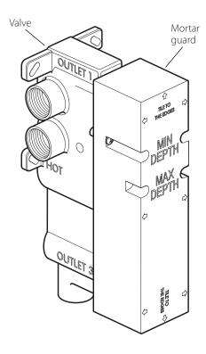
Rinse pipe work thoroughly before fitting the valve: do not allow dirt, metal particles or shavings to block the filters fitted on inlets.
