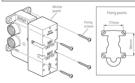
Select the position for the shower valve and offer the shower valve to the wall, make sure the valve is vertical with a level and mark the 4 fixing points with a suitable pencil, see above right for dimensions. Remove the shower valve from the wall, drill the holes to a suitable depth for the wall plugs and secure with suitable screws.
