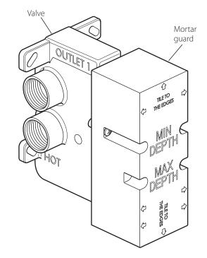
Rinse pipe work thoroughly before fitting the valve: do not allow dirt, metal particles or shavings to block the filters fitted on inlets.
