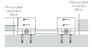
Connect the  ${\bf hot}$  and  ${\bf cold}$  water supplies to the 3/4" BSP fittings at the bottom of the valve body
