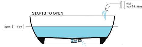
At a depth of 25 cm the Smartwaste gradually starts to open, until the waste fully opens above a depth of 36 cm.
