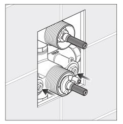
Turn off both non return valves by turning clockwise, do not overtighten.
