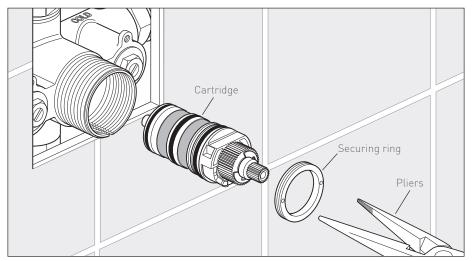
**Important:** ensure the hot and cold water supplies have been isolated. Using a pair of long-nosed pliers unscrew the securing ring and remove. Pull the cartridge out from the body
