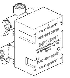
**Valve body** (with mortar guard)
