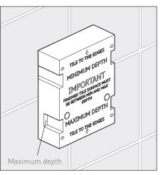
Finish the wall by tiling up to the mortar guard, keep the final finished wall surface between the min and max marks.
