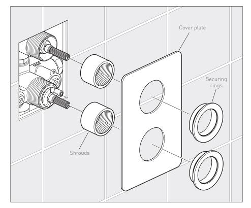
Screw shrouds on ensuring they sit proud of the finished wall. The shrouds can be turned/adjusted to achieve this.
