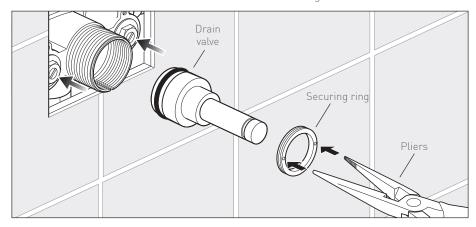
Close both non return valves. Remove the speedfit connector. Using a pair of long-nosed pliers unscrew the securing ring and remove. Pull the drain valve out from the body
