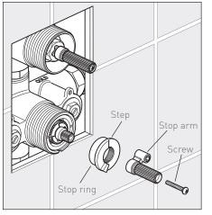
Remove the screw from the temperature stop arm and pull off. Pull off the stop ring (note the position of the step).
