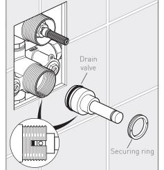
Push drain valve into the body, replace the securing ring and tighten.
