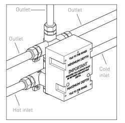
Use the supplied adapters if required. Connect hot supply to the lower left inlet of the valve and cold supply to the lower right inlet. Connect the top and bottom outlets to the desired channels.
