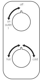
Turning the bottom handle anti-clockwise will increase the water temperature.
