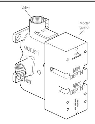
Rinse pipe work thoroughly before fitting the valve: do not allow dirt, metal particles or shavings to block the filters fitted on inlets.
