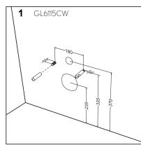
1. Install installation frame in accordance with manufacturers instructions. Set out as detailed to the left
