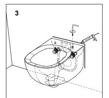
3. Locate the WC on the fixing studs and using the key provided securely tighten each wall fitting.
