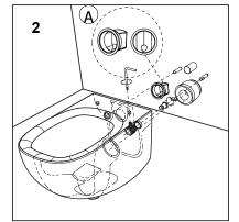
2. Fit wall fixings into the WC as shown. Ensure the flat section on the fixing stud point upward.
