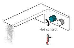
Turn the control clockwise to increase the flow of hot water
