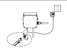
Connect the IR sensor from the tap to the control box. If necessary, according to the product version (AC or AC+DC), power the system via the transformer socket.
