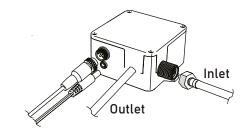
Install filter elements and connect the water inlet and outlet securing with clip.
