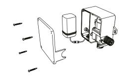
According to the product version, (DC or AC+DC), open control box and remove the battery box.
