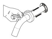
Make the holes in the wall, pass components through the main hole and secure spout with appropriate components. Slide wall plate from the front and secure threading it to spout assembly.
