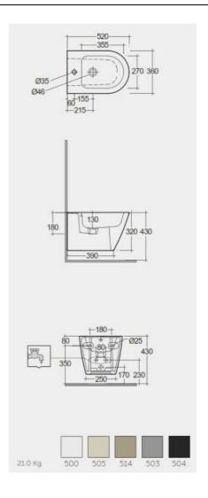
Dimensions: All dimensions in mm. Tolerance of vitreous china & fireclay items:  $\pm$  5% for below 200mm and  $\pm$  3% for above 200mm; for all other items tolerance  $\pm$  1%. Note: Due to a continuing development program to improve design and performance, the manufacturer reserves all rights to vary specifications without prior information. Please note accessories are for photographic use only.
