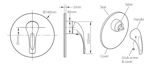
Remove the backing paper from the seal on the back of the cover. Slide the cover over the valve, push onto the wall until it makes contact.
