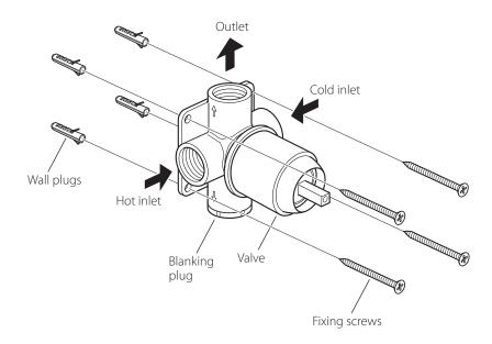
Before installing your new mixer, flush through the pipe work to ensure removal of debris, turn off the water supply.
