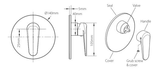
Remove the backing paper from the seal on the back of the cover. Slide the cover over the valve, push onto the wall until it makes contact.
