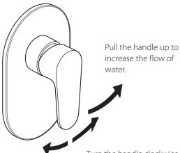
Turn the handle clockwise to increase the temperature and anti-clockwise to decrease the temperature.
