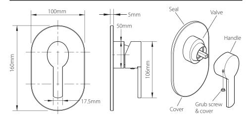
Remove the backing paper from the seal on the back of the cover. Slide the cover over the valve, push onto the wall until it makes contact.
